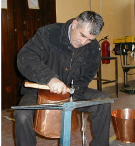
Thomas Keenan constructing a copper bucket
